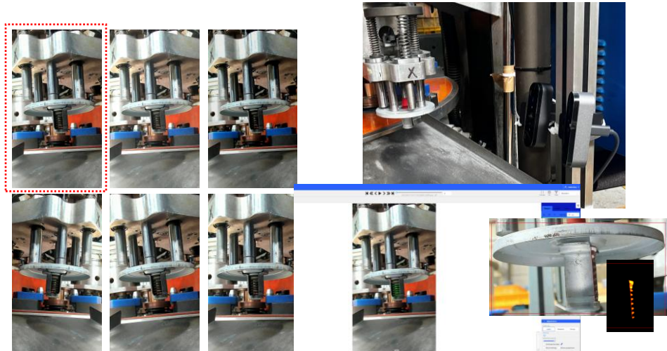
(Left) Original + 5 augmented images (Top right) Camera installation scene (Bottom right) Labeling interface and sample result
